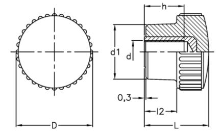
$$\begin{array}{ll} D & = 26 \\ d1 & = 16 \\ d \ 6H = M6 \\ h & = 16 \\ L & = 28 \\ I2 & = 15 \end{array}$$
